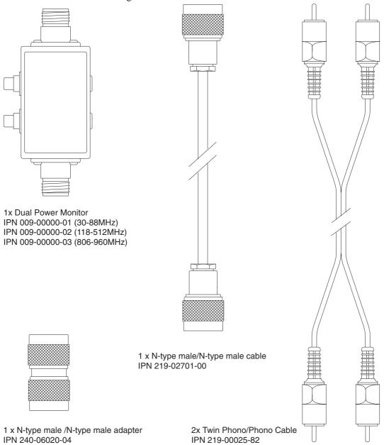
More details of the cables follow in the Wiring Specifications section.
